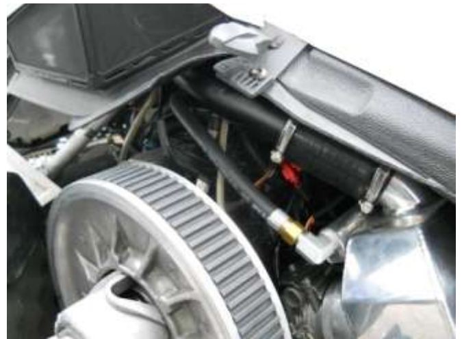
The long leg of the fuel line gets screwed onto the fuel rail.
