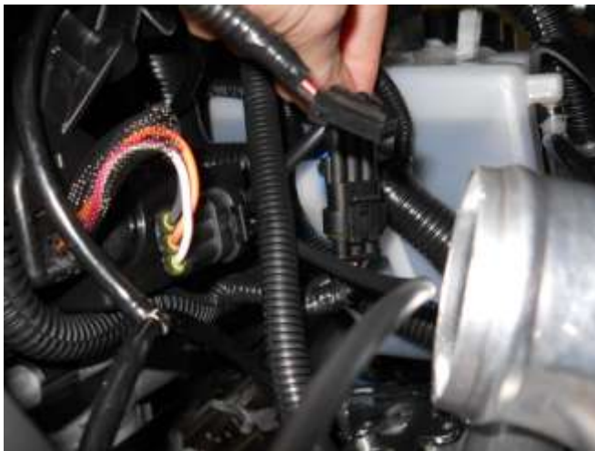
Unplug the ignition coil plug, this is directly across from the fuel rail and is pictured above. The Aero-Commander harness gets connected inline at this plug.
