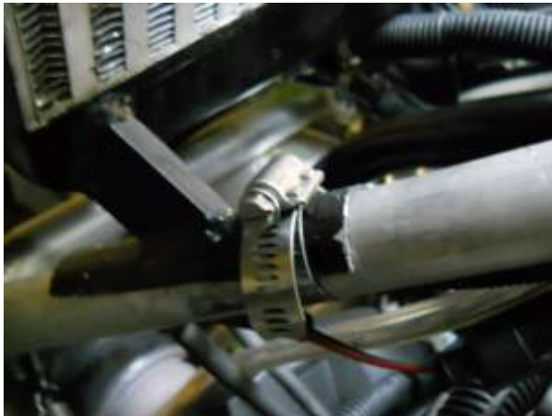
Tighten the clamp around the intercooler bracket to secure the intercooler to the chassis.
