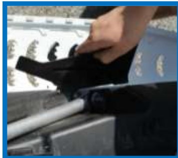
On either side of the gas tank, midway down, there are two 13mm nuts covered by panels that snap off. Pull outward on the panels to remove them.
