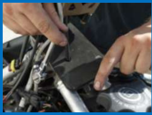
Two 10mm bolts connect the frame members running along the gas tank to the handle bar neck.
