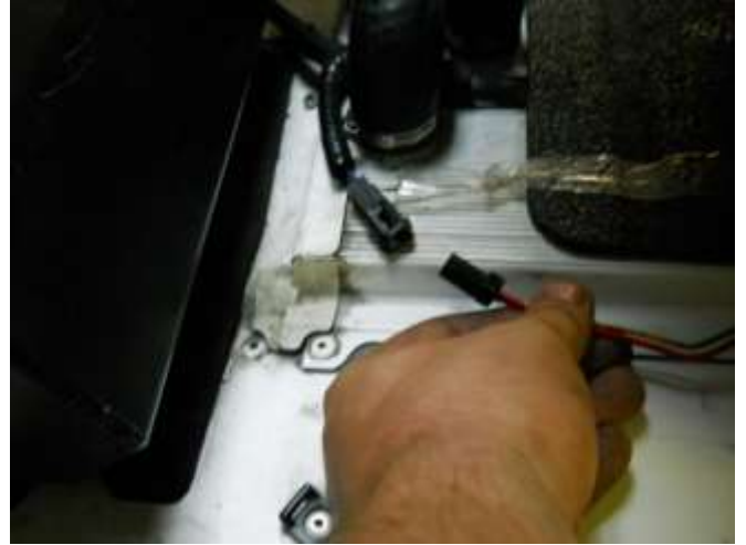
Re-connect the plug coming off the bottom of the tank.
