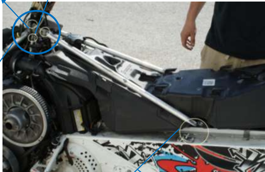
There are two vertical members attached at the handle bar neck connected with two 10mm bolts.
