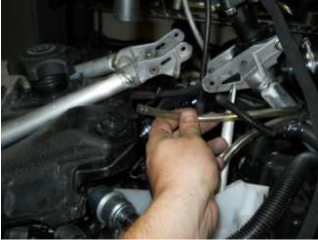
Re-connect the breather line at the top of the tank.
