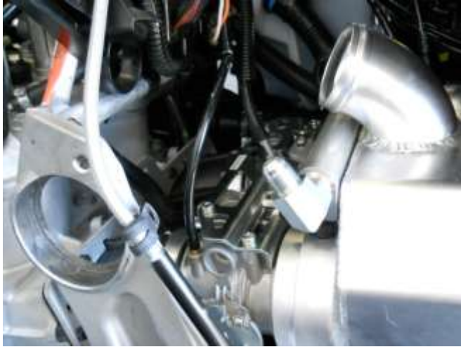
The signal lines that are labeled “to manifold”, get attached to the hose barbs on the throttle bodies.
