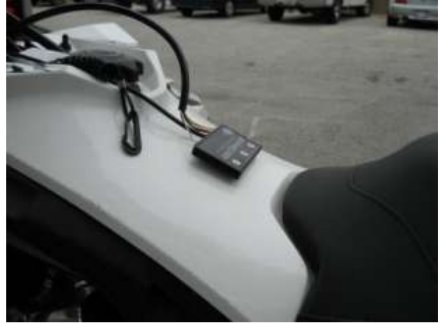
The line labeled “to Aero-Commander” gets routed to the handlebars and will be connected to the Aerocommander later when it is installed.
