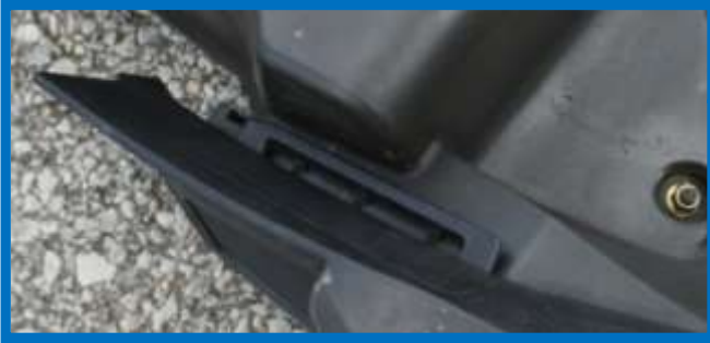
There is another snap tab at the bottom the vent.
