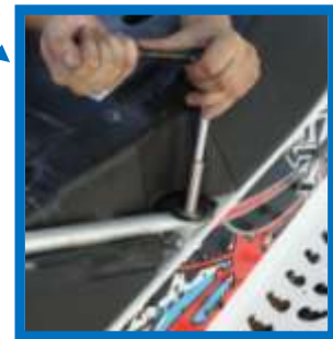
Use a 13mm ratchet to remove the nuts on both sides of the gas tank.
