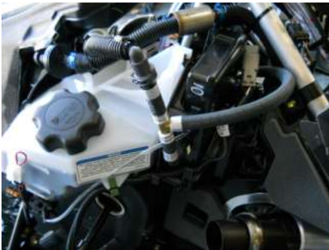
The short legs of the line get installed between the gas tank fuel line and the ECU.
