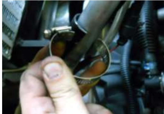
Wrap the hose clamp around the intercooler and chassis and reconnect it to itself.
