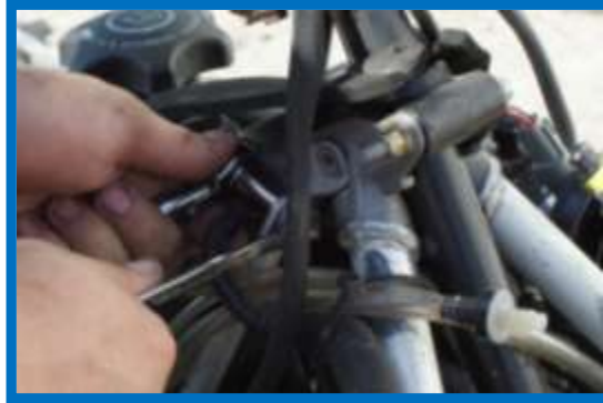
There are two vertical members attached at the handle bar neck connected with two 10mm bolts.
