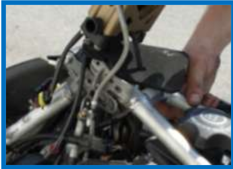
Remove the four 10mm bolts and the frame members over the gas tank will be loose from the handlebar neck.
