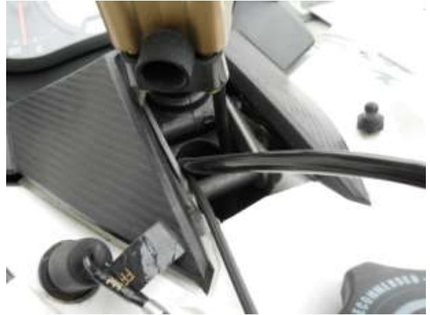
Run the electrical harness through the handlebars and into the sled.
